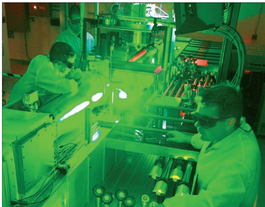
Berkeley researchers (Wim Leemans, left and Csaba Toth, right) assisted by technician Joe Wallig (back) are aligning a high-peak-power laser system, TREX, that is used to power laser plasma accelerators in the giga-electron-volt class. (Courtesy Berkeley Lab.)
